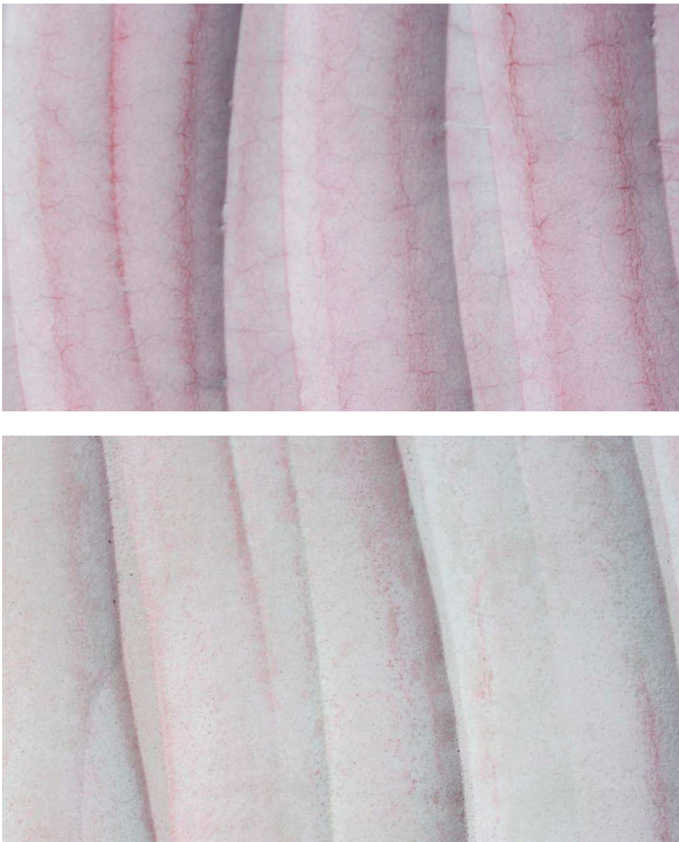
Figure 4. Pictures of GRC panels produced with textured molds and made without polymer modification (4A) and with 6% Forton polymer solids (4B). Surfaces were treated with a red dye solution to highlight any face cracking.
